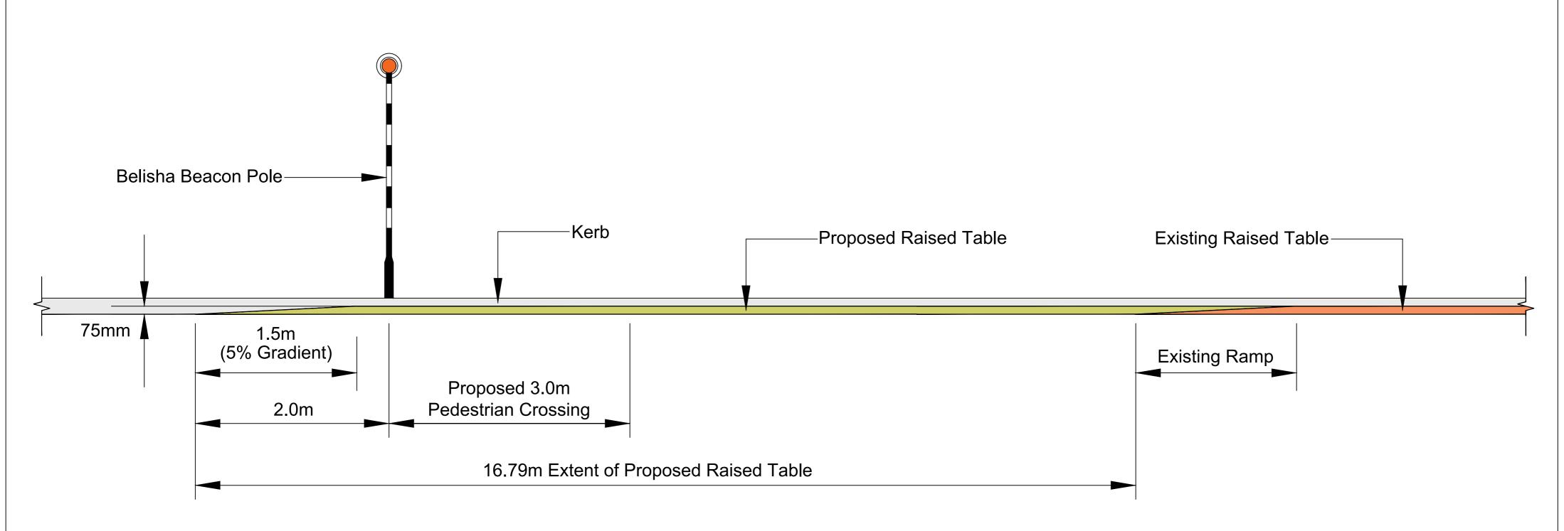
SECTION C-C (LONGITUDINAL SECTION THROUGH RAISED TABLE)
