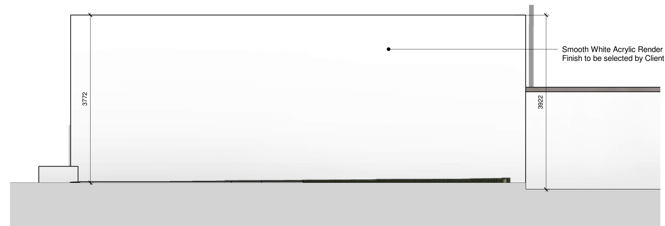
3 North West Elevation
