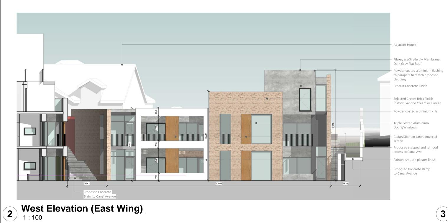
Selected Cream Brick Finish -Ibstock Ivanhoe Cream or similar Formica Vivex Panels F6067 Steel Materia or similar Friple Glazed Windows with Aluminium Cills breglass/Single ply — Membrane Dark Grey Flat Painted Smooth -Plaster finish Cedar/Siberian Larch louvered screens 1.2m Steel Balcony -Railings Plaster bead detail between windows Opaque Glazing to Wet rooms Doors with vision panel
