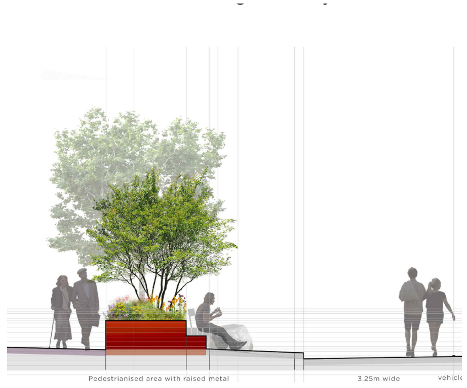
Section B-B through raised planter with seating
