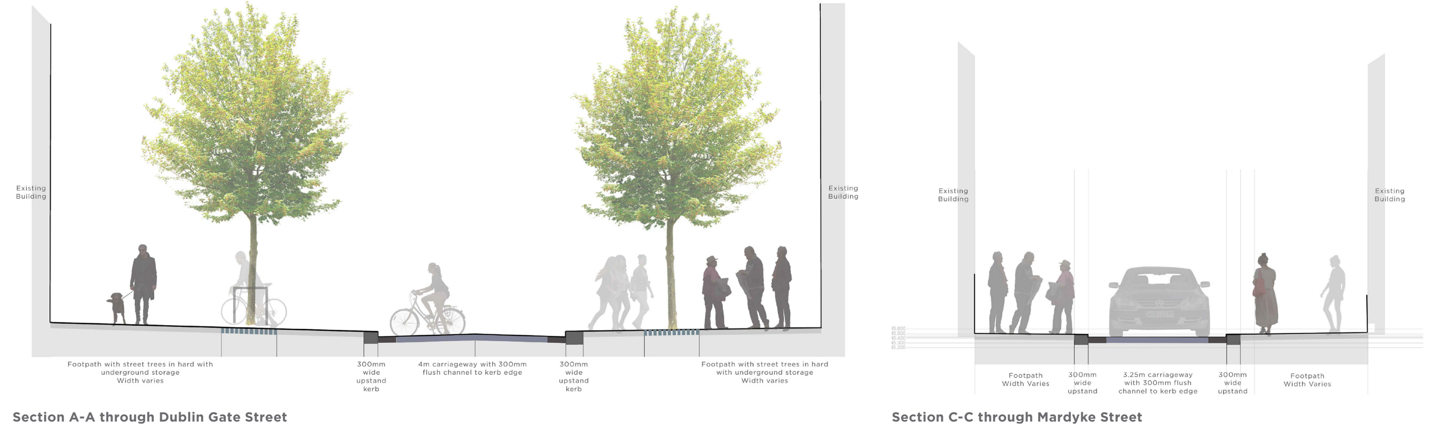
Section A-A through Dublin Gate Street
