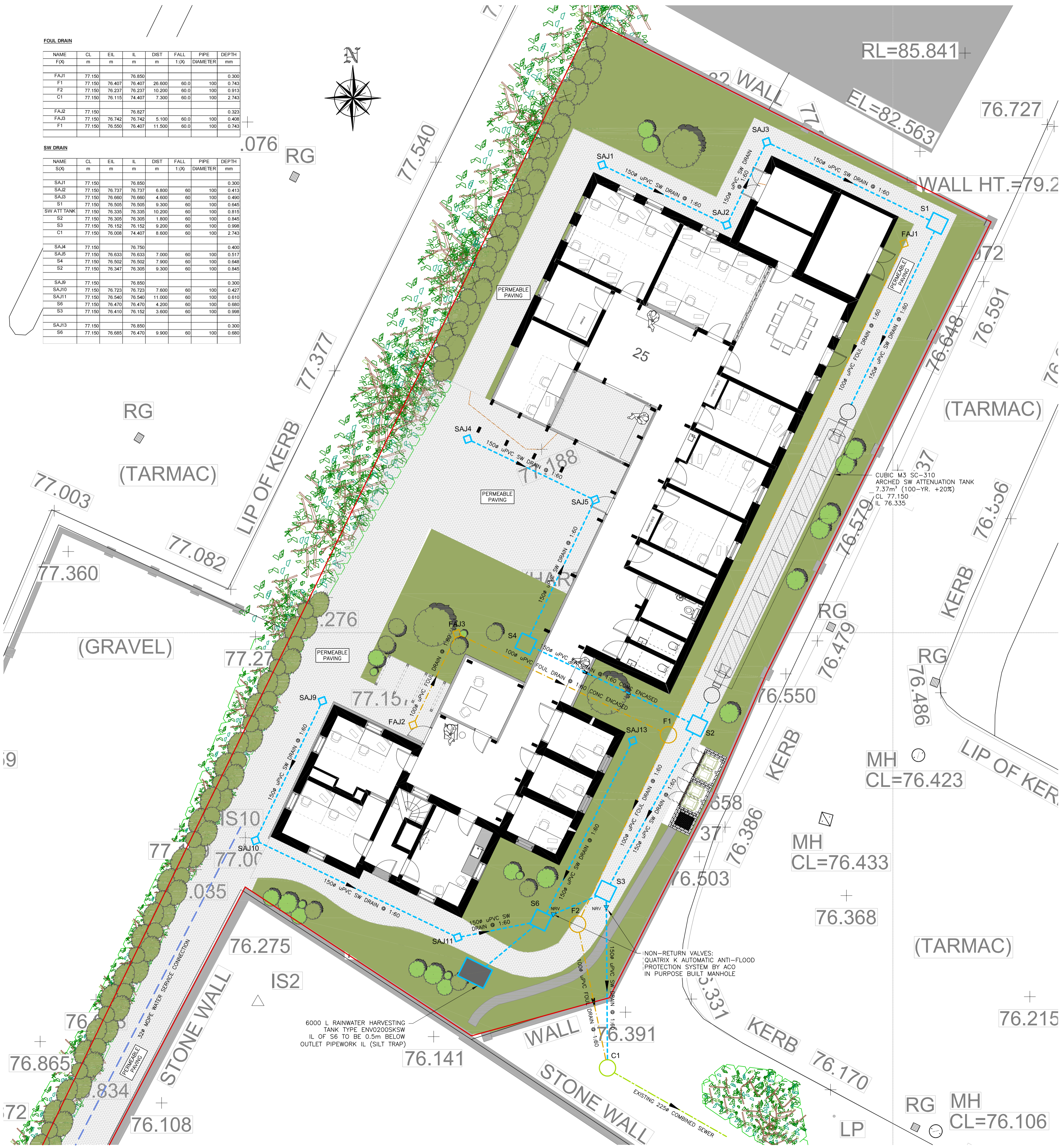
SITE LAYOUT PLAN - DRAINAGE
