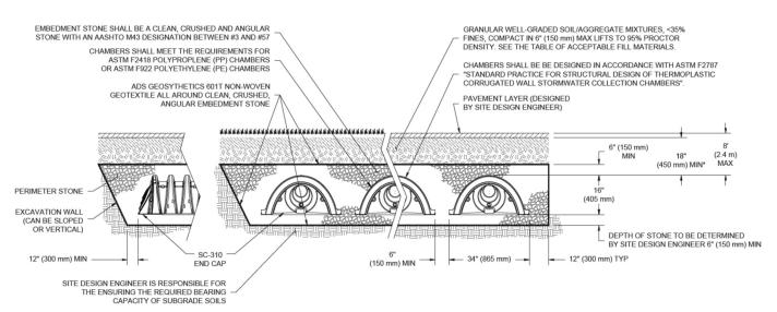
\*MINIMUM COVER TO BOTTOM OF FLEXIBLE PAVEMENT. FOR UNPAVED INSTALLATIONS WHERE RUTTING FROM VEHICLES MAY OCCUR, INCREASE COVER TO 24" (600 mm)
