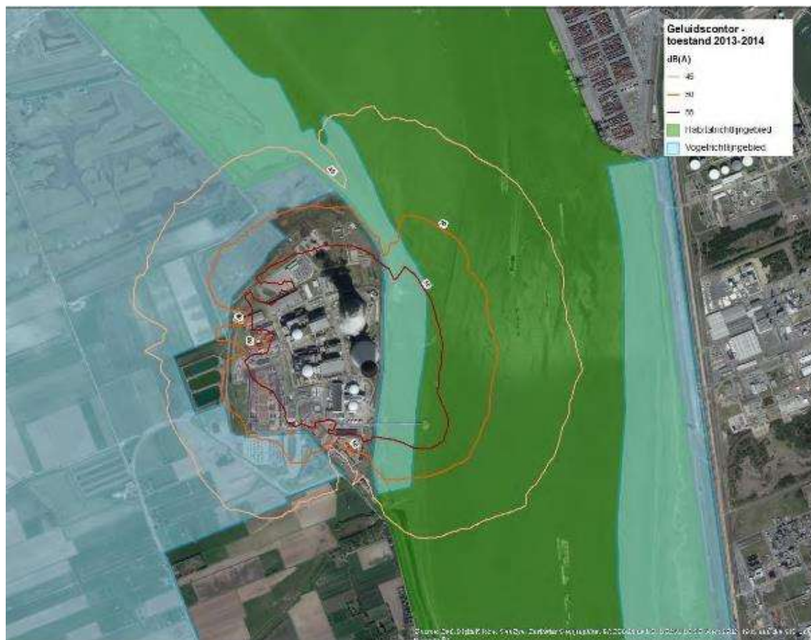
Figure 45: Noise contours of the continuously operating sources during the day, evening, and night periods (Source: EIA Arcadis/NRG, 2021).
