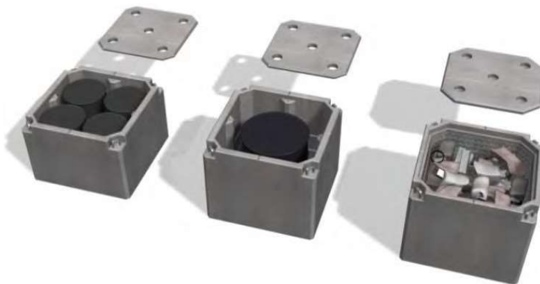
Figure 27: Illustrations of the three types of caissons lvi containing waste: type I (left), type II (center) and type III (right). After placing the lid and filling the space between waste and caisson with filler mortar, these disposal colli are called "monoliths."
