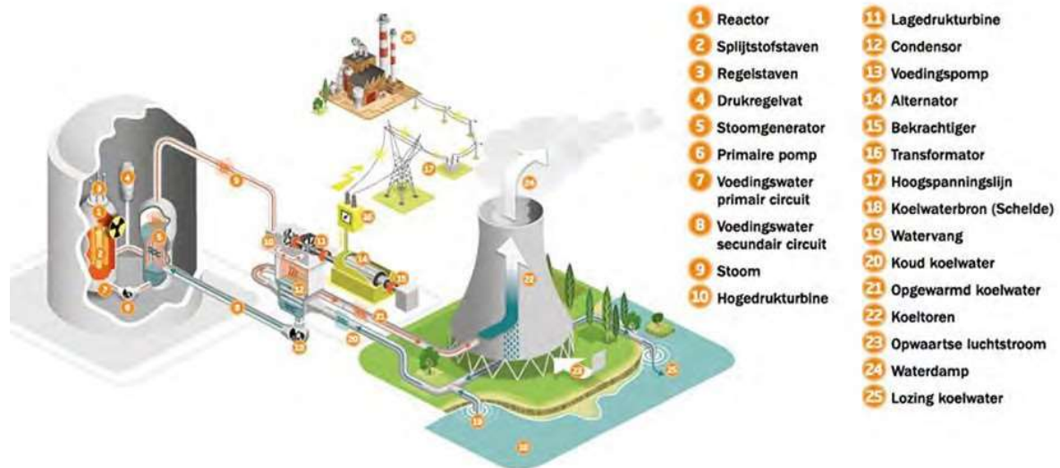
Figure 2: Operation of nuclear power plant with reactor building, engine room and cooling circuit from left to right (Source: Electrabel nv).
