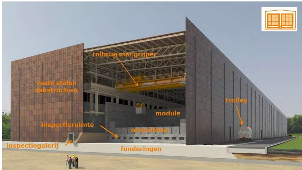
Figure 28: Sketch of the repository for category A waste during backfilling with monolithslvii .
