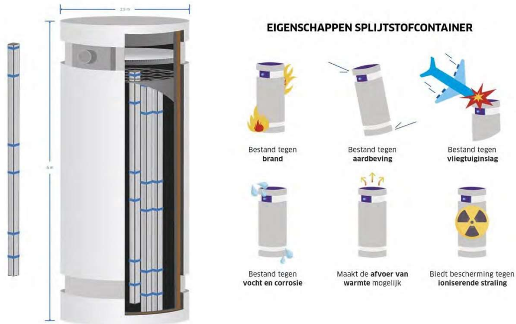
Figure 26: Principle of dry storage of spent fuel elements in Dual Purpose Casks (DPC) as provided in the SF2 storage facilities lii . The packaging consists of a metal structure designed to allow the residual heat of the spent fuel to be passively dissipated by internal conduction, radiation and natural convection. The package is made of metal and other materials that provide protection from ionizing radiation.
