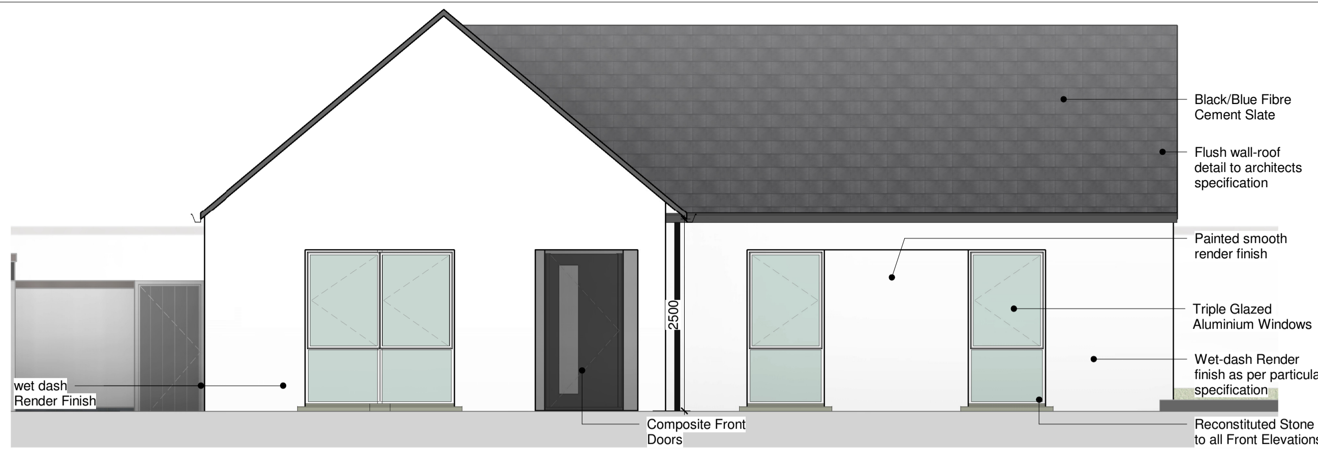
3 South West Elevation
