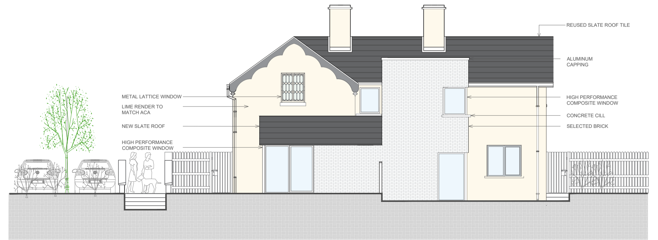
REAR ELEVATION Extended Matrons House SCALE 1 : 100 @ A1
